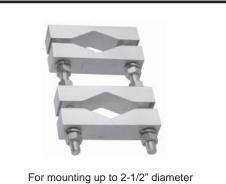
For mounting up to 2-1/2" diameter antenna to a 2-1/2" maximum diameter mast (2 per assembly).
